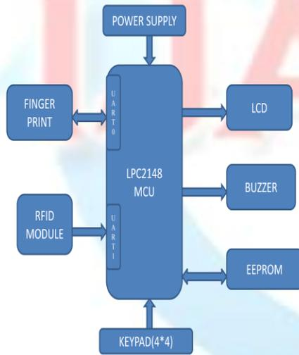
Fig 5: Block diagram of the system.
