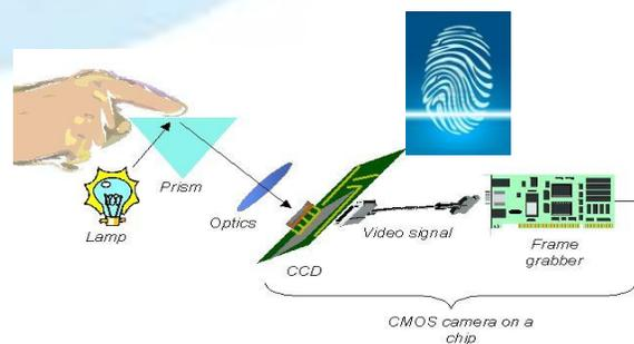
Fig 3: Finger print optical reader Reflection diagram.
