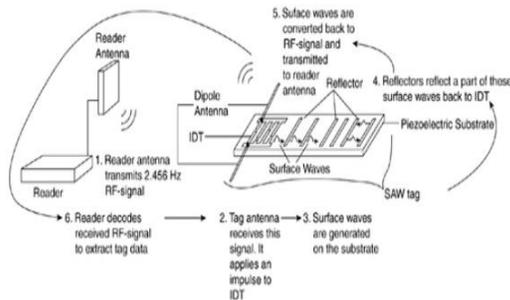
Fig 2: RFID Communication process
