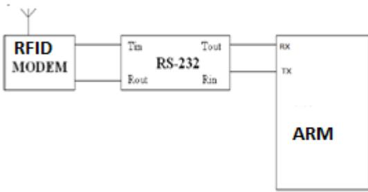
Fig 1: Interfacing RFID module with controller
