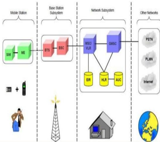
Fig.2: Architecture of GSM network
