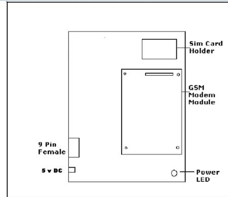
Fig 1. GSM Modem Block Diagram.
