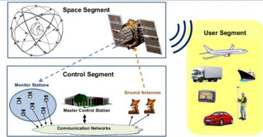
Fig.2: Architecture of Gps network
