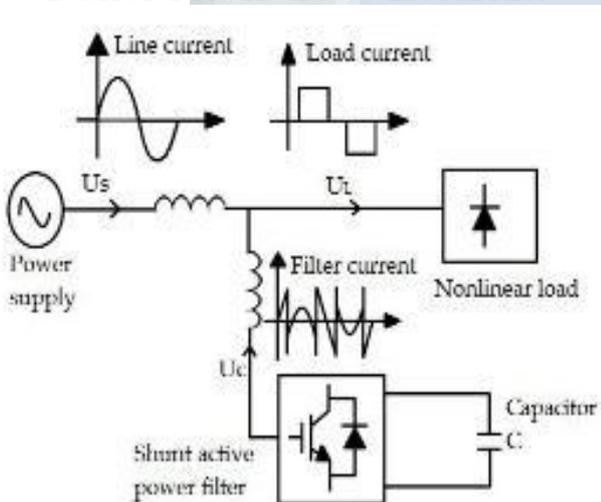
Fig.2 Schematic of Shunt active power filter
