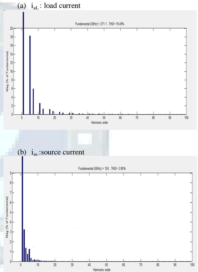
Fig.7 Harmonic magnitude in load and source currents
