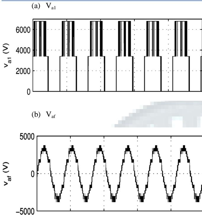
Fig.8 Reactor terminal and output voltages
