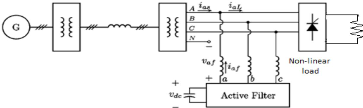
Fig.1 Active filter connection to a shipboard power system
