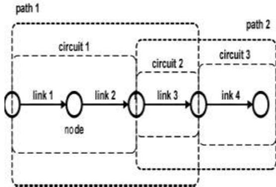
Fig. 1. Model structure in terms of nodes, links, circuits, and paths.
