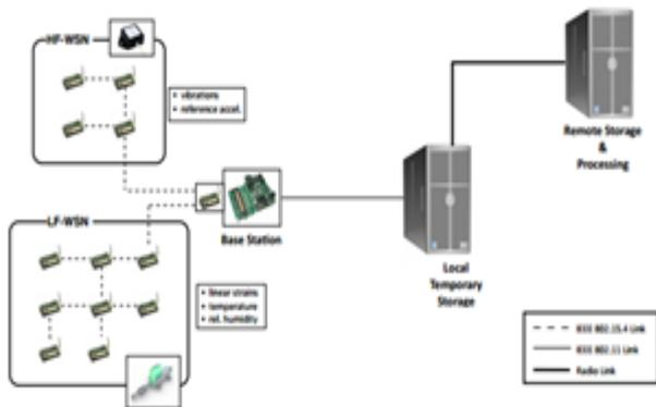
Fig. 1. A schematic description of the architecture of the proposed system
