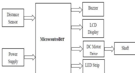
Figure shows block diagram of the system. Description of the hardware is given below. Microcontroller is performing all calculations and controlling all output devices such as buzzer, LCD display, DC motor and LED strip. Distance sensor is an input device.
