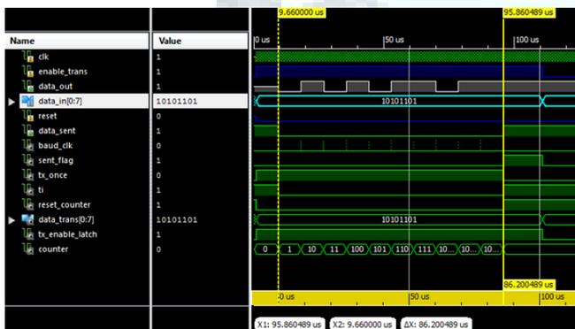
Fig. 5 Simulation Results for UART transmission
