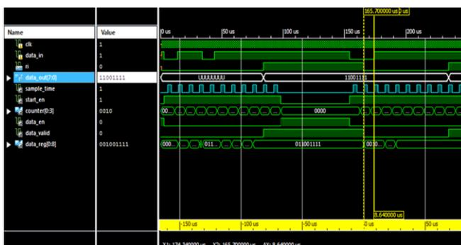
Fig. 6 Simulation Results for UART reception
