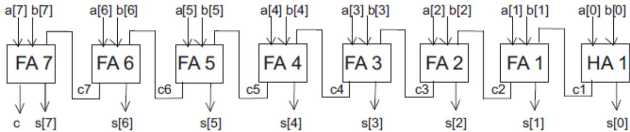
Figure 6. Block Diagram of ADDER1.
