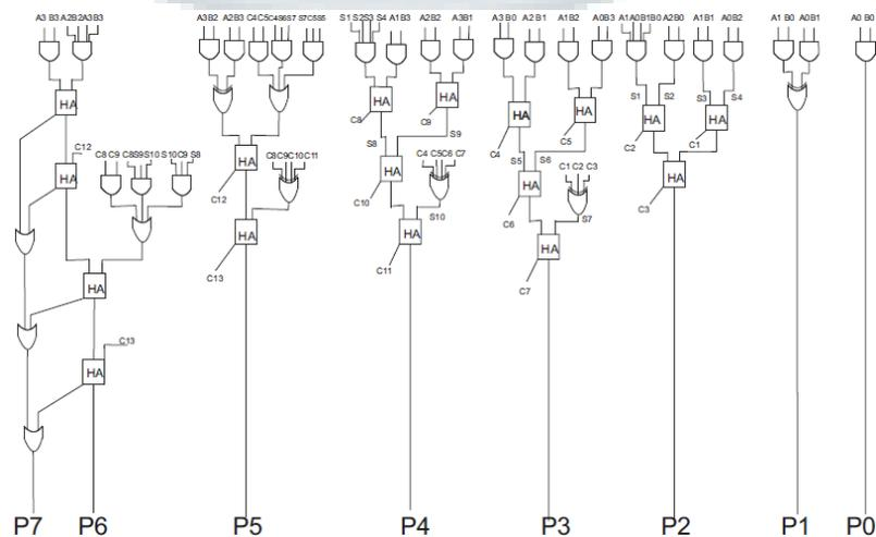
Figure 5. Gate Level description of modified 4-bit multiplier.
