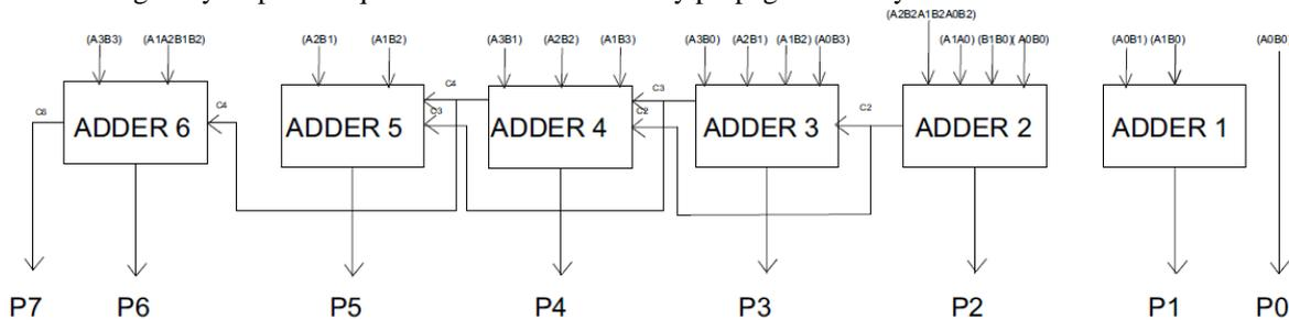
Figure 4. Proposed 4-bit Vedic multiplier using Urdhva Tiryagbhyam sutra and carry-skip technique.
