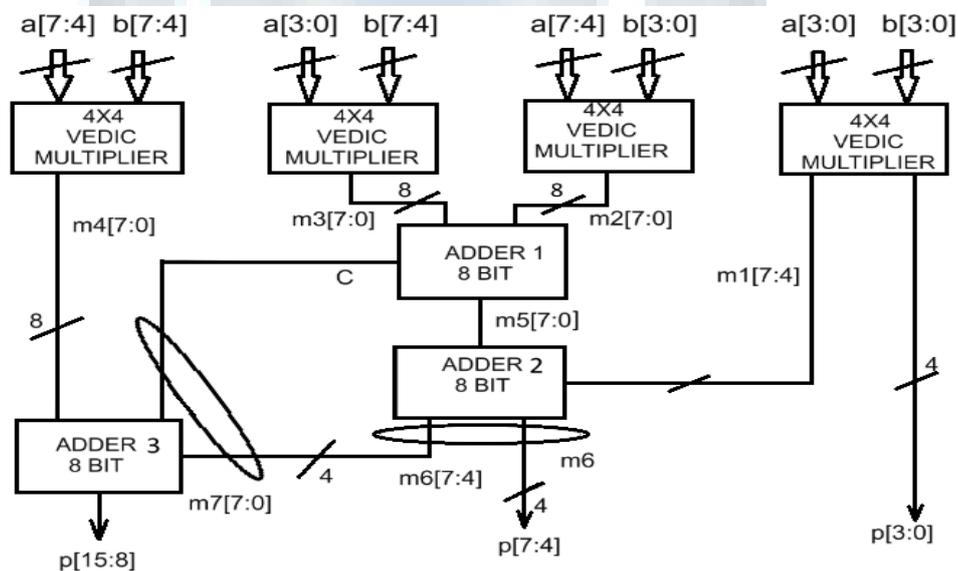
Figure 2. Block diagram of proposed 8x8 multiplier.
