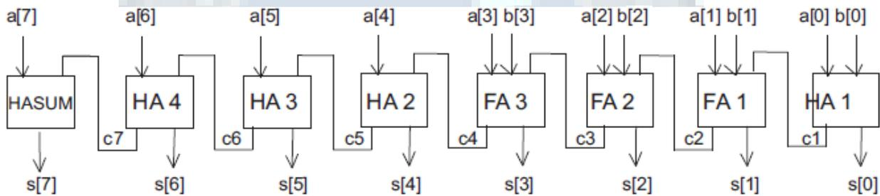
Figure 7. Block Diagram of ADDER-2
