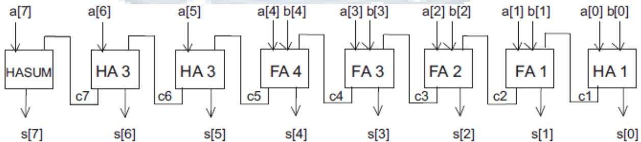
Figure 8. Block Diagram of ADDER-3
