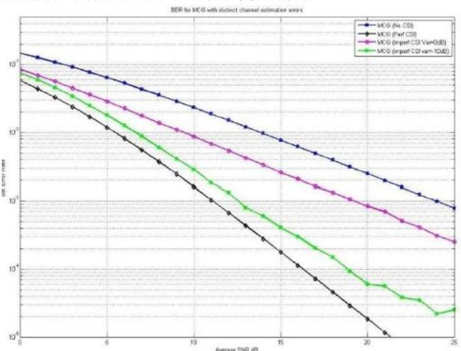
Fig 8: Comparison of MCG with distinct channel estimation
