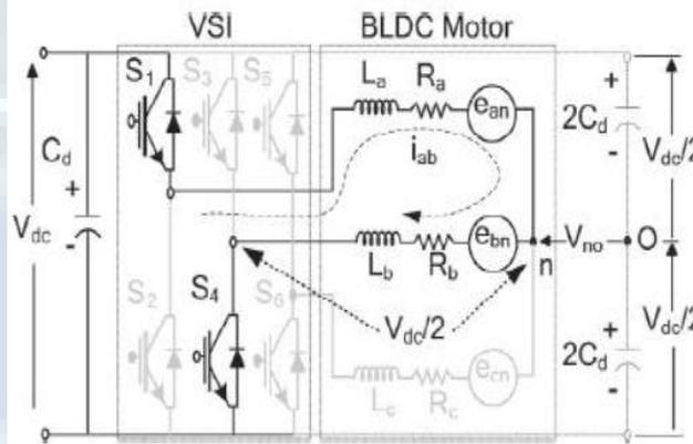
Fig.3. Operation of a VSI-fed BLDC motor when switches S1 and S4 are conducting.
