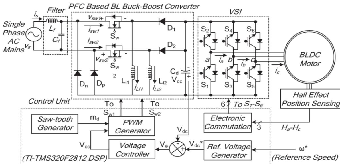
Fig. 1. Proposed BLDC motor drive with front end BL buck- boost converter.
