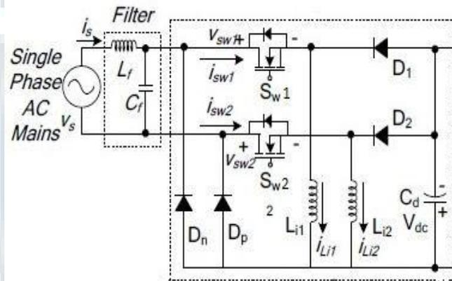
Fig. 2 PFC based bridgeless Buck-Boost Converter
