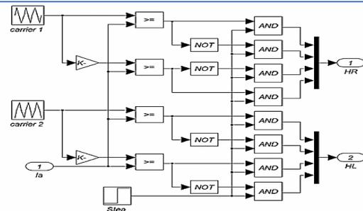
Fig 3. Gating Signal Generation by PSCPWM
