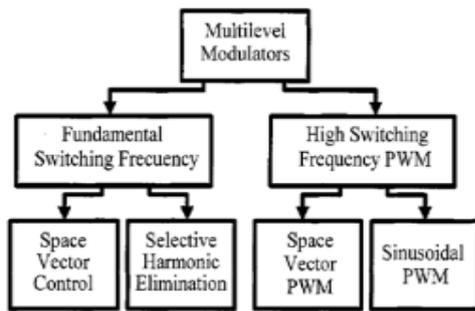
Figure.5:Classification Of Multilevel Modulation Methods.
