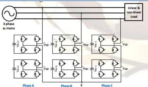
Fig. 2. Cascaded Multilevel Inverter
