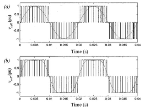
Figure.6: Inverter Cell Voltages. (A) Output Voltage And Reference With SPWM.(B) Output Voltage And Reference With Injection Of Sinusoidal Third Harmonic.
