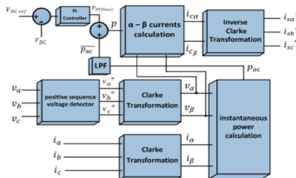
Fig 4. Control block diagram for reference current generation
