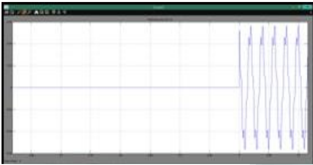
Fig:7.13 d -axis fault components of the rotor current for a voltage dip down to 60% under condition of the typical second-order system.
