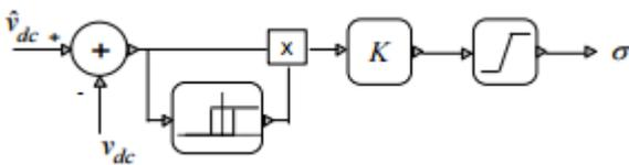
Fig. 3. Central dc voltage controller at offshore MMCs.
