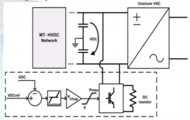
Fig.4. Control scheme of onshore dc chopper resistor.
