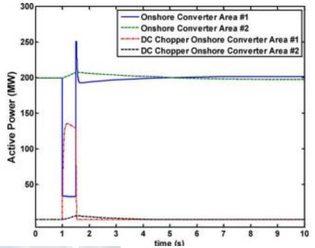
Fig9. Onshore converter and dc choppers active power
