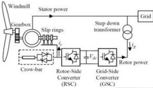
Fig. 2. Schematic diagram of a DFIG wind turbine.
