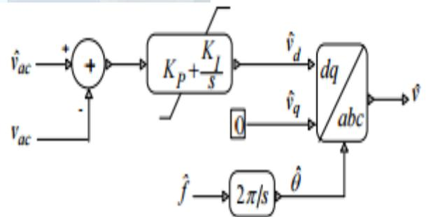
Fig. 1. Offshore MMC control.
