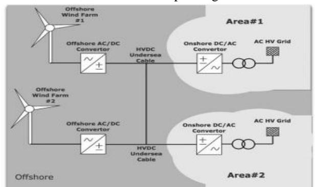
Fig.6. MTDC grid test system.
