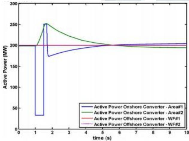
Fig7. Active power flows on HVDC–VSC.
