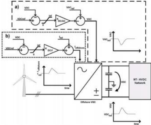
Fig5. Control scheme for FRT provision based on dc voltage: (a) AC offshore grid voltage control. (b) AC offshore grid frequency control.
