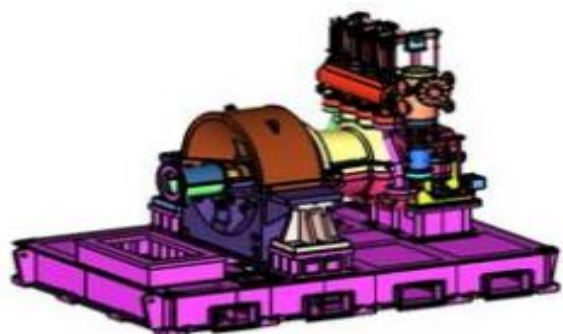
Fig 1:10MW Steam Turbine Overall Assembly
