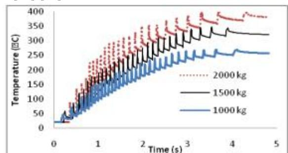
Fig. 5. Effect of different vehicle masses on disc temperature
