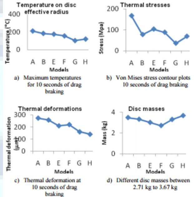
Fig. 14. Drag braking analysis
