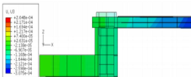
Fig. 8. Disc coning at the end of stop (4 s)
