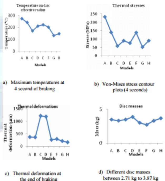
Fig. 11. Single stop braking analysis
