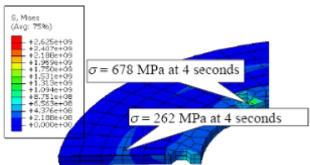
Fig. 7. Thermal and mechanical stress contour plot for the 1000 kg vehicle mass
