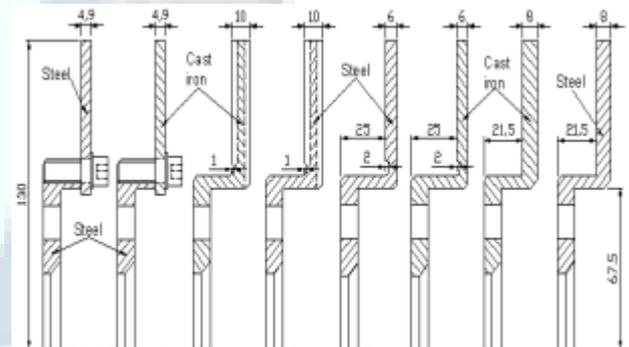
A 3.48 kg Gi-B 3.32 kg Gi-C 3.48 kg Ss-D 3.87 kg Ss-E 3.01 kg Gi-F 2.71 kg Gi-G 3.30 kg Ss-H 3.67 kg
