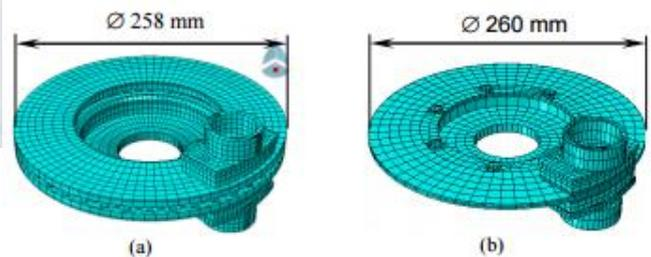
Fig. 1 (a). Standard ventilated disc (total mass is 5.71 kg) (b) Prototype disc (total mass is 3.48 kg)
