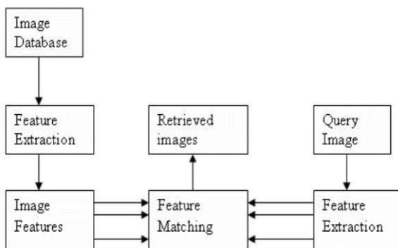
Fig. 1. Block diagram of CBIR system
