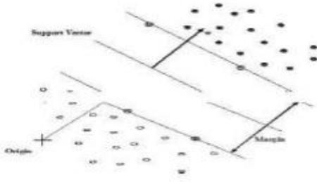
Fig. 3. Linear separating hyper-planes for two class separation.
