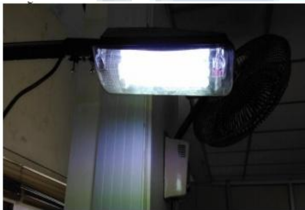
Fig 7: Status of the Light is ON after obstacle detection
