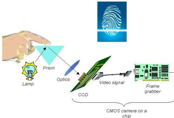
Fig 3: Finger print optical reader Reflection diagram.
