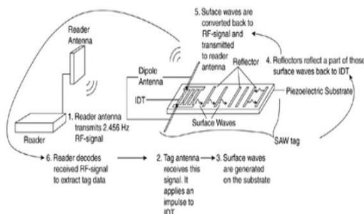
Fig 2: RFID Communication process
