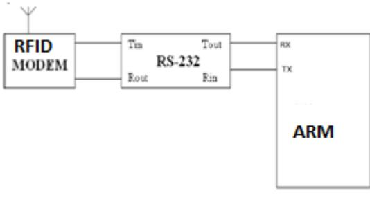
Fig 1: Interfacing RFID module with controller
