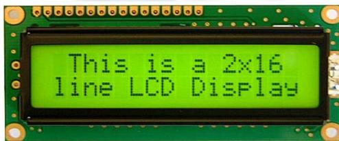
Fig8. 2x16 LCD display
