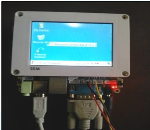
Fig12 (a): ARM9 as transmitter section
